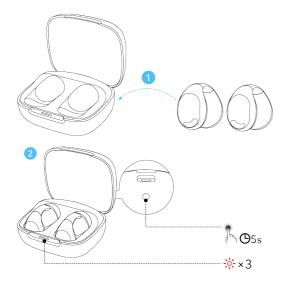
Place the earbuds in the charging case and leave the case open. Press and hold the charging case button for 5 seconds until the LED indicator flashes red slowly three times.
