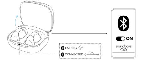
Open the case to power on the earbuds and enter pairing mode. Select "soundcore C40i" from your device's Bluetooth list.
