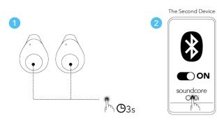
Method 1: Manual Pairing with the Second Device While wearing the earbuds, press and hold the intuitive button on both earbuds for 3 seconds until you hear a voice prompt of entering pairing mode. Then you can proceed to pair with the second device. Please note that if you attempt to connect a third device, the earbuds will automatically disconnect from the first device, as the earbuds can only connect to a
