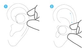
1. Hold your ears with one hand, and gently clamp the earbuds onto the upper part of your auricles. Make sure the front side faces your ear canal and the back side with intuitive button rests behind your ear. 2. Move the earbuds upwards or downwards until the earbuds fit securely and you can hear the sound well.
