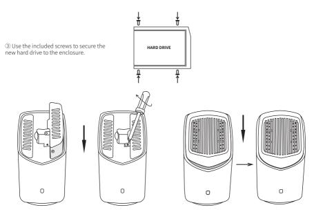
② Insert the enclosure back into the H1 HomeStation and tighten the screws, then put the top cover back in place. You can expand your storage room after cutting off power to the HomeStation by following the steps above. The new hard drive must be initialized through the Baseus Security APP for use with the H1 HomeStation.
