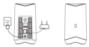
1 Turn on the H1 HomeStation and connect it to your router. When the LED light turns blue, it means the H1 HomeStation is ready for setup (this will take approximately 1 minute).
